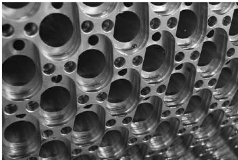
Figure 4. Detail from outer rotor surface. The couple of cavities above cell and duct are for bolts.
