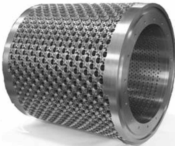
Figure 5. Rotor without closings (almost 500 kg of pure titanium, 60 × 73 cm ( \text{\O} \times \text{H} )).
