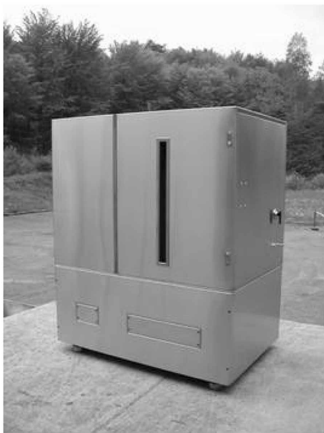
Figure 1. The Partitron 25 hydrostatic preparative chromatograph, 1.5 m (L) \times 1 m (D) \times 1.85 m (H), weight: 1,200 kg (control panel not shown).
